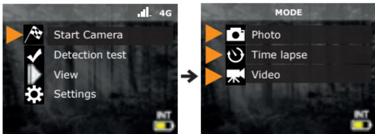
Click on Start Camera and select the desired operating mode (photo, time lapse or video) in the Mode menu by pressing OK. If you start the camera in Video mode, make sure that you have enabled the Photo First setting.
