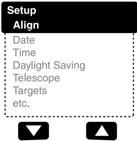
Fig. 15: Menu options display on the second line. Use the Scroll keys to move up or down through the list of options. Press ENTER to select the desired option.
