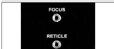
Fig. 58: 14" model auxiliary focus and reticle jacks are located on the inner left fork arm.
