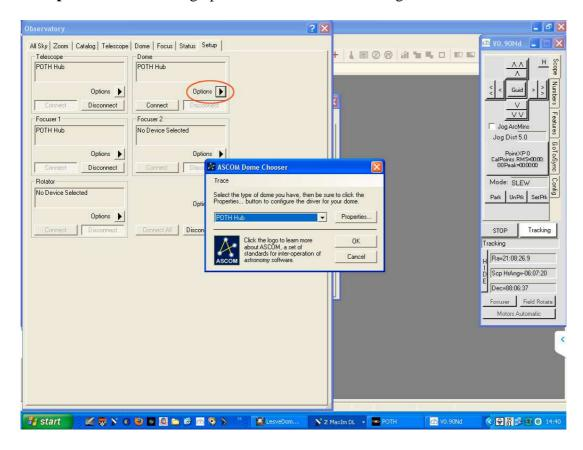
Next, click on the **Properties** button and fill in the slaving information from your spreadsheet into the 'Geometry' section in the Metric units shown.
