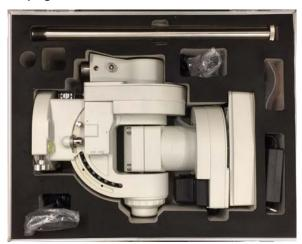
2. Attaching the Mount: The mount has a 150mm diameter base which can be mounted onto an optional iOptron 2" tripod or pier. There are two sets of mounting studs and azimuth locking nuts.
