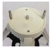
Remove the alignment peg from a iOptron tripod/pier if it comes with one. Thread the two studs
