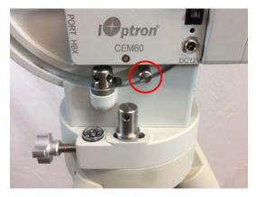
3. <u>Setting the Latitude:</u> Slightly loosen the Latitude Locking Clamps, use the SS lever if needed.
